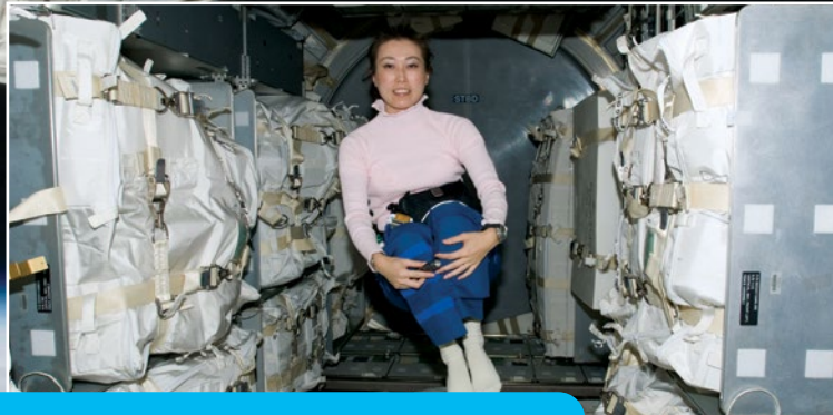
During construction, supplies were delivered using the Multi-Purpose Logistics Module, or MPLM. The MPLM launched in the shuttle's cargo bay. Once docked to the ISS, astronauts could go inside and unload the cargo. Here is Japanese astronaut Naoko Yamazaki inside the MPLM.
